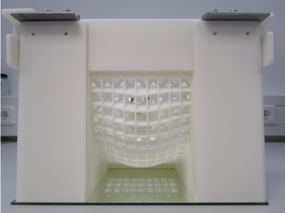
Figure 5.6.2: Mirror positioned underneath the base of the test apparatus (Front view).
