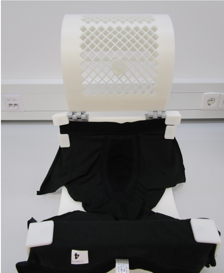
Figure 6.1.2: Demonstration of garment placement on test specimen and the use the magnetic clips to lock the garment in place (top view).
