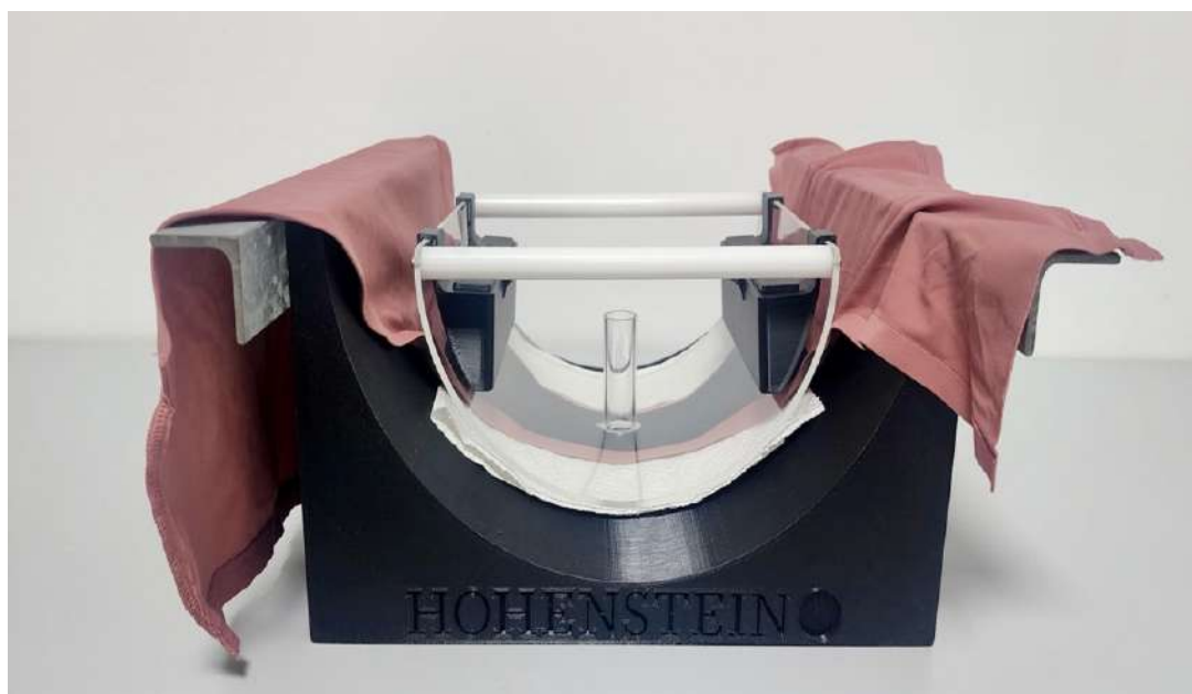
Figure 6.8: Test setup with female reusable absorbent undergarment.
