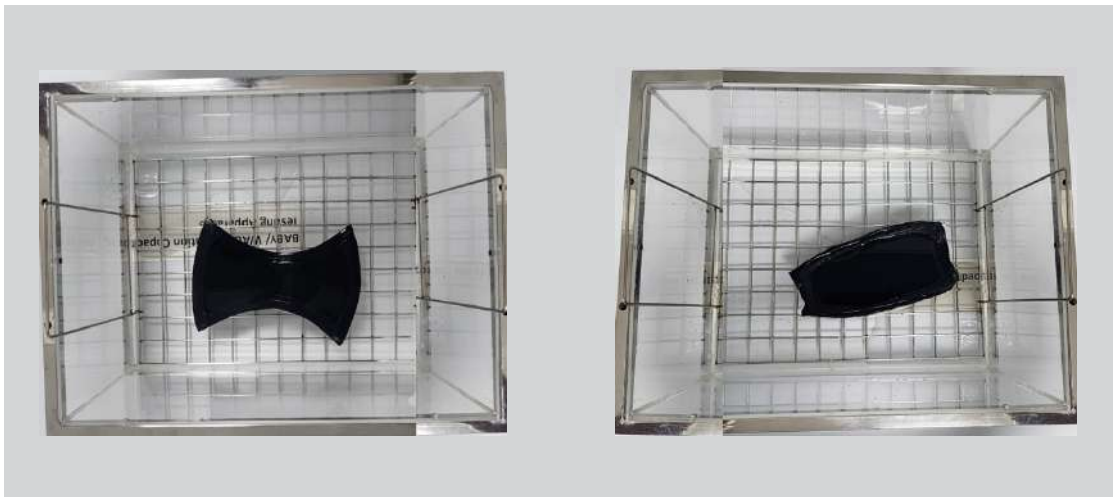
Figure 7.2.1: Cut & separated absorbent gusset (left) & absorbent pouch (right) submerged in the saline solution bath (top view).
